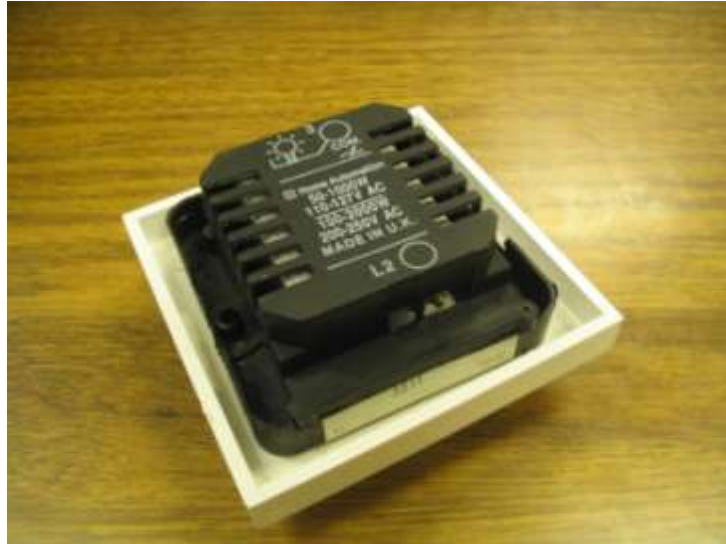
Figure 3.11 Continuous Transformer from back
