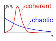
The photo-count distribution in this graph is obtained experimentally by letting the light fall on a photo-detector through a shutter that is open for a very short interval. And counting the number of photons registered by the photo-detector. This measurement is repeated many times and a time delay is allowed between successive measurements. This delay should be long compared to the coherent time of the light.
